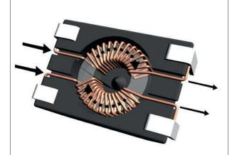
When the common mode component of a signal tries to go through the choke, it will meet a high impedance, due to the inductance created by the magnetization of the core and the coils.
