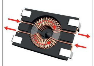
In opposition to the common mode behaviour, the differential mode component of the signal will see almost no impedance in the choke, this phenomenon could be explained with the magnetic field compensation inside the core. If the core is not magnetized, then no inductance will appear in the line.
