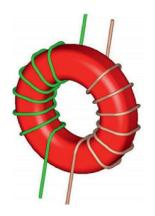
**Sectional winding:** Shows the highest attenuation in differential mode. This chokes are recommended for power lines, where a high isolation is mandatory and the power delivery is happening at low frequency.
